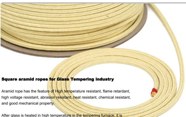
After glass is heated in high temperature in the tempering furnace, it is quenched rapidly by the wind grid, and then transferred onto series metal rollers which are spirally wrapped by aramid ropes. As the glass is still hot, aramid ropes can effectively protect the hot glass from contacting the low temperature metal rollers and without cold explosion and no scratch.
