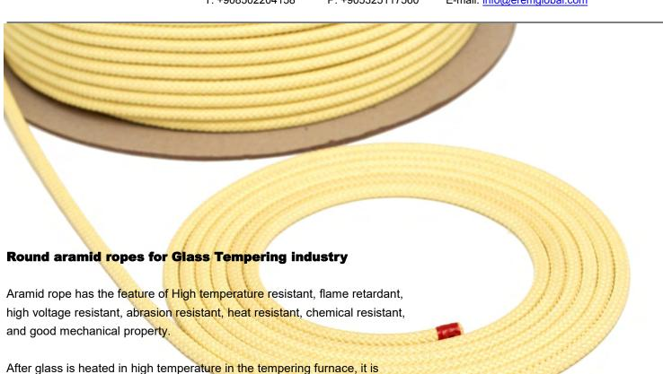
After glass is heated in high temperature in the tempering furnace, it is quenched rapidly by the wind grid, and then transferred onto series metal rollers which are spirally wrapped by aramid ropes. As the glass is still hot, aramid ropes can effectively protect the hot glass from contacting the low temperature metal rollers and without cold explosion and no scratch.
