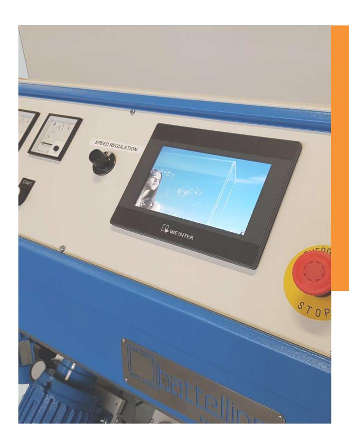
All working phases can be controlled from the PLC
